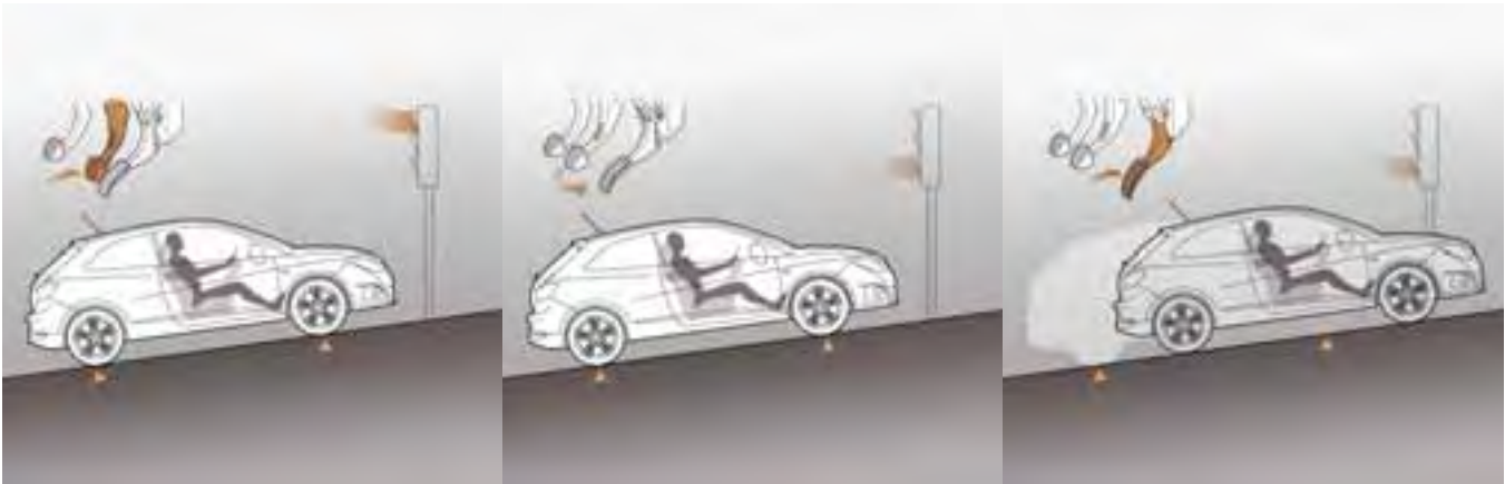
Hill Hold Control applies the brake for two seconds, making hill starts easier.
