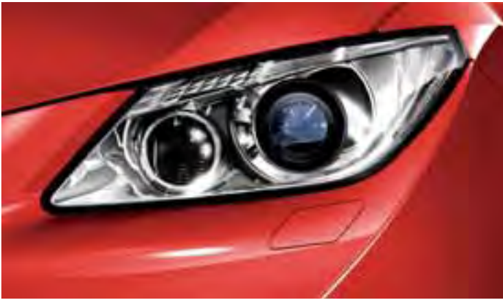
Bi-xenon headlights with AFS (Adaptive Front-lighting System).
