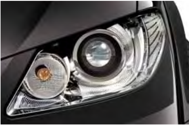
Bi-xenon headlights with AFS, headlight washer system and daytime running lights.
