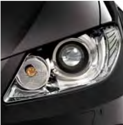
Bi-xenon headlights with AFS, headlight washer system and daytime running lights. SE Sp
