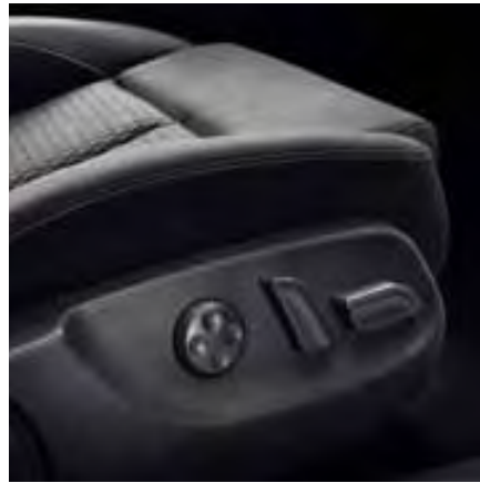
Twelve-way electric front seats and memory function for drivers seat (up to 4 positions, part of Electric Seat Pack). SE Sp
